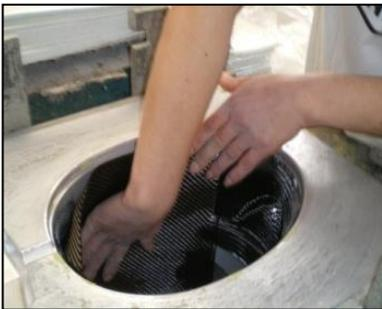
This operation must be carried out with high precision and care, as it determines the quality of the final helmet .
