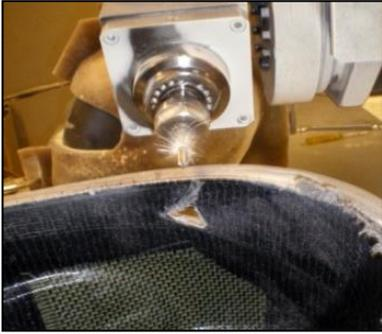
The window and the holes of the row shell are milled. The last production phase of the shell is that of grinding and then the painting with paints that have a low coefficient of linear thermal expansion in order to avoid cracking over time.
